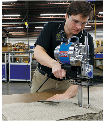
▲ Eastman Machine Company President Trevor Stevenson demonstrates the power and precision of the Blue Streak Straight Knife cutting through multiple layers of textile fabric.
